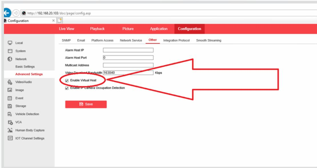
Enable the “Virtual Host” setting to allow visibility of all cameras connected to the POE switch on the NVR.
