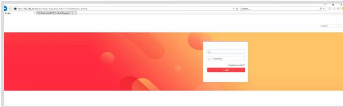
Enter the IP address of the NVR into Internet Explorer to access the web interface. The default user-name will be "admin" with the password that was previously setup with the SADP tool.
