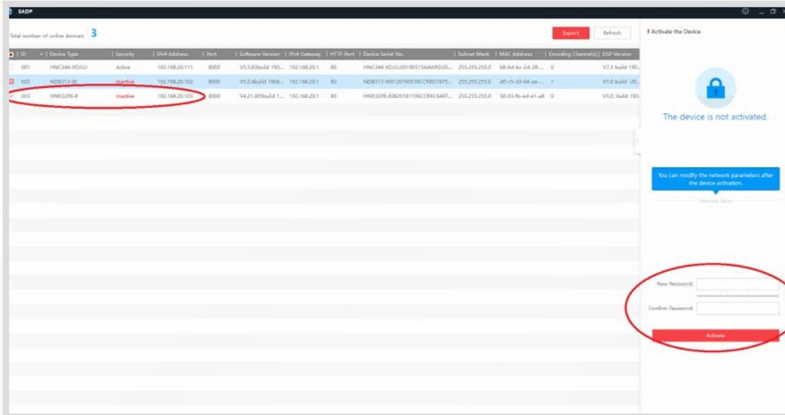
Open the SADP Search tool and locate the PAV NVR. In the right side panel, enter the desired password for the NVR. This password will also be sent to any cameras currently connected to the POE ports on the rear, as well as any future cameras connected to the POE ports of the NVR.
